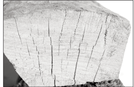
Dry Firewood will show “checking” or cracks at the end of the split
